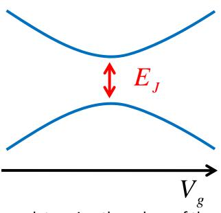
We now discuss the various conditions necessary for this system to be a viable qubit (1)<u>Initialization</u> is achieved simply by applying a sufficient bias and allowing sufficient time for the system to come to thermal equilibrium. Since the values of  $E_J$  and  $E_C$  are typically of order1 K, while to eliminate quasiparticles T must be <80 mK, in equilibrium only the lower energy eigenstate is occupied.
