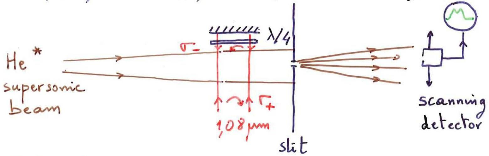
$$\text{Interaction time} = \frac{33 \text{ mm}}{1100 \text{ m/s}} = 30 \mu\text{s}$$
