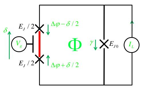
The « quantronium » design solves this problem by adjusting, between the qubit operation and the readout, not the qubit Itself but a « distant » element of the circuit. With the notation shown in the figure, the Hamiltonian of the qubit (the red area) is
